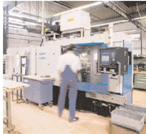
It has been a year of investment at Franz Funke. Precision components, e.g. for the automotive industry, are produced on this CNC-controlled 6-spindle automatic lathe.
